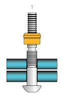
The pin is inserted into the prepared hole and the smooth bore collar is placed on the pin.
