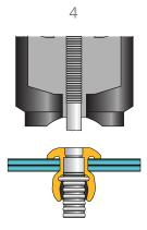
A solid circle lock between the pin and sleeve is formed just prior to the pin breaking flush with the sleeve head, completing the installation.
