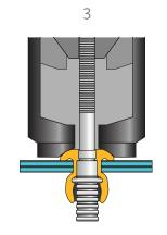
Continued pulling on the pintail expands the sleeve to maximum allowable diameter. As the shear ring reaches the backside of the work piece it breaks and catches on the tapered annular grooves, keeping high pressure on the blind side of the work pieces as the pin continues to draw down inside the sleeve.
