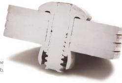
Lock groove on pin engages shoulder on rivet head, while the support ring "double locks" the pin within the bulb.
