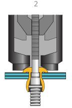
Insert the fastener into the hole and slip the installation tool over the pintail. Press the trigger to initiate pulling action. As the tool pulls on the pintail, the shear ring feature on the pin pulls inside the sleeve fully expanding the diameter and drawing the work pieces together.
